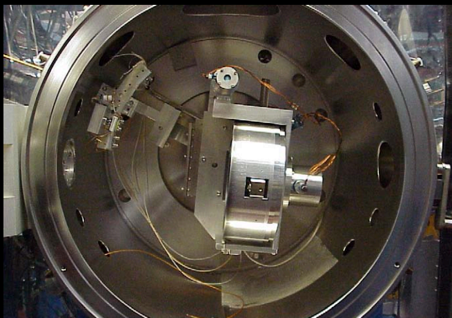
(far left) CXRO Reflectometer's monochromator grating. (left) The reflectometer's vacuum chamber. (upper left) The MET's secondary mirror.
